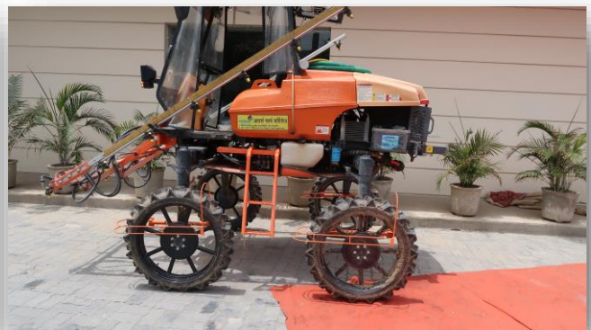
Tractor sprayers are good for PPR/PRE spray (L), but not preferred by farmers for narrow row spaced crops, the new machine imported from Japan by UPL is very effective for POE herbicides spray (R)
