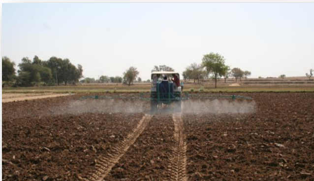
Tractor sprayers are good for PPR/PRE spray (L), but not preferred by farmers for narrow row spaced crops, the new machine imported from Japan by UPL is very effective for POE herbicides spray (R)
